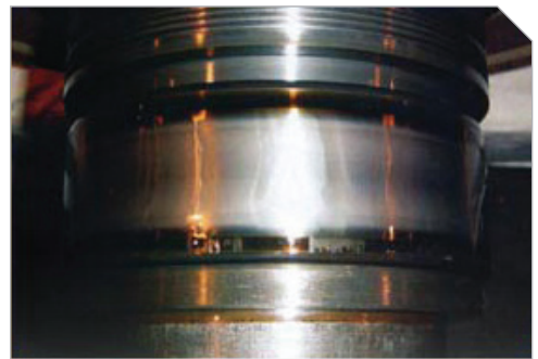
FIGURE 5 - Inner race of same NU326 greased bearing after disassembly.
