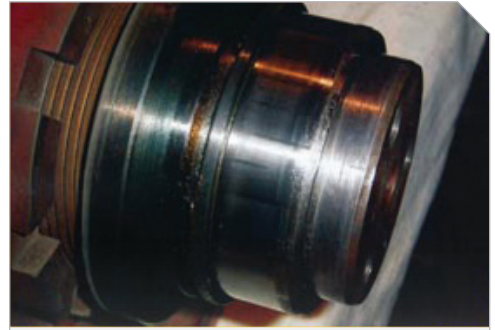
FIGURE 4 - NSK #NU326 280mm oil-lubricated bearing after more than 80,000km of high-speed service.
