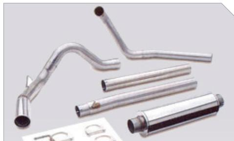
Our second test was to install a Magnaflow turbo back exhaust system. Mileage increased by just seven tenths of a percent, but power increased by 6.2 percent.
