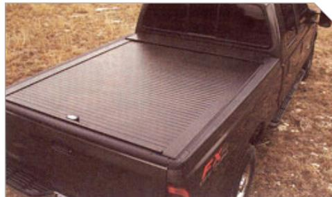
This American Roll cover was installed at Truck Covers USA. The resulting improved aerodynamics gave us another 1.56 mpg.
