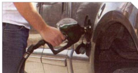
For our mileage testing, we drove the test course at 67 mph, keeping rpm between 1900 and 1950, then topped off again. Our baseline was 17.2 miles per gallon.
