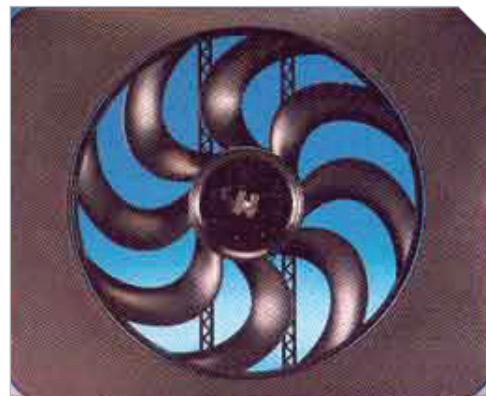
Whether you are using a mechanical fan or electric, a shroud will greatly increase its efficiency in terms of how much air it actually pulls through the radiator core. This Flex-a-lite electric fan comes with a built-in shroud — just make sure it covers at least 70 percent of the radiator's surface area.
