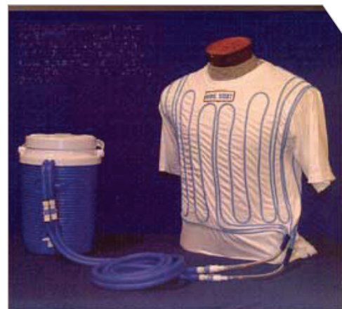
Most cool suit designs feature several feet of surgical tubing sewn into a shirt that is worn next to the driver's skin. A small electric pump pushes chilled water through the tubes, cooling the driver.
